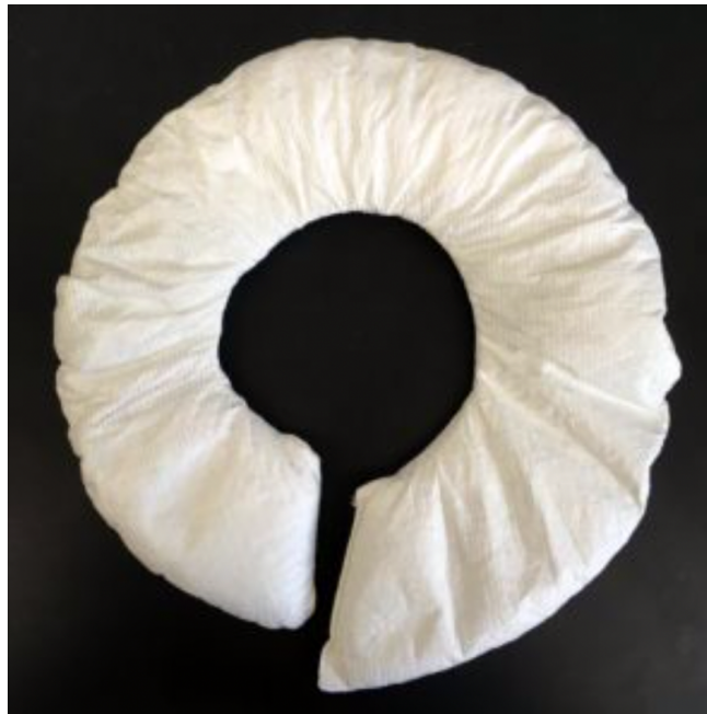
This is an example of a simple support you can create to place around the base of statues. It is made from Tyvek (used in building construction and easy to find in local markets) and filled with sand or other weight .
